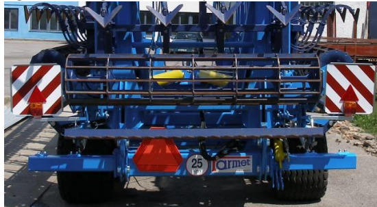
Fig.18 – Placing the rear safety shields
