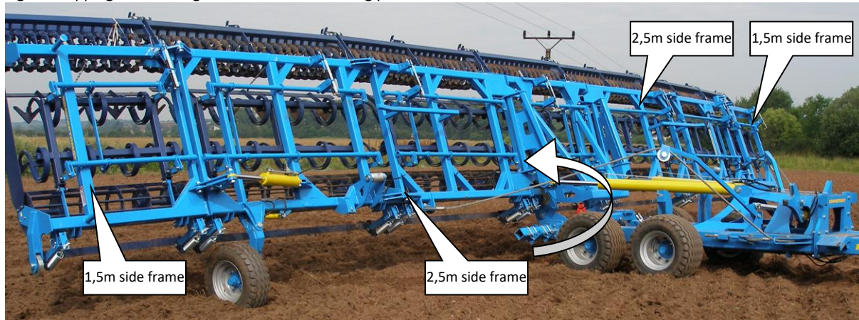
Fig.13 – Tipping the working section into the working position
