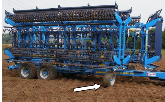
Fig.10 – Auxiliary wheels are prepared for unfolding
