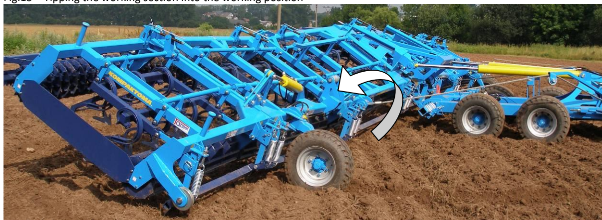
Fig.13 – Tipping the working section into the working position
