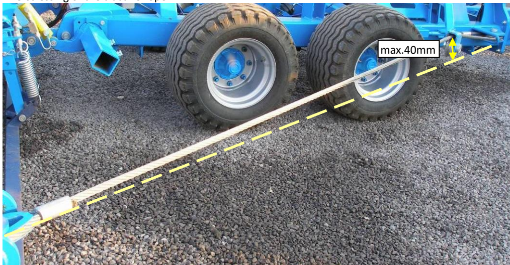
Fig.24 – Pre-stressing of the tractive rope
